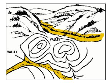
Contour lines forming a ridge tend to be U-shaped or V-shaped. The closed end of the contour line points away from high ground.
